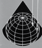
Distances along meridians and standard parallels are correct. Shapes and areas are distorted.
