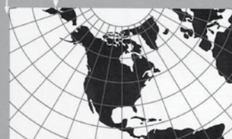
Equal areas. Deformation of shapes increases away from standard parallels.
