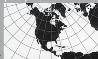
Large-scale map sheets can be joined at edges if they have same standard parallels and scale.
