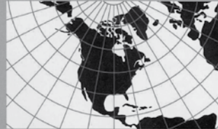
Distances along meridians and standard parallels are correct. Shapes and areas are distorted.
