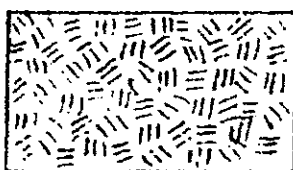
ASBESTOS OR FIBER
