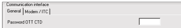
Fig. 19: Protect the OTT CTD with a password – input window to establish a password.
