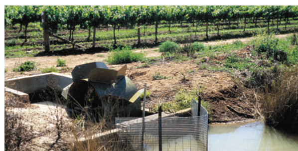
d. Dethridge wheel measuring irrigation water consumption by vineyard, Griffith, NSW. (Source: CSIRO. By: Willem van Aken on 8 November 1995)
