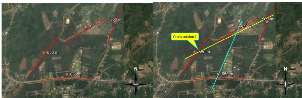
Fig. 5. Vertical electrical sounding (VES, 1D) surveys in the study area and south of it: left: location of center, line direction, and max. AB/2 in meter; right: location of cross section 1 shown in Fig. 6.
