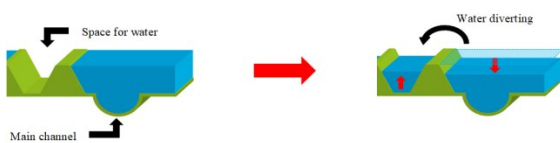
Fig. 2. Operation of high water channel Source: (roomfortheriver.nl, n.d.)
