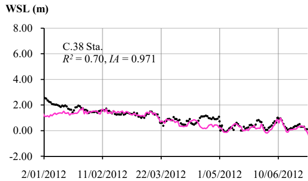
Fig. 6. Comparison of time series of stage hydrograph between simulated results (smoothed-line) and measured data (dotted) at the major gauge stations (model verification).
