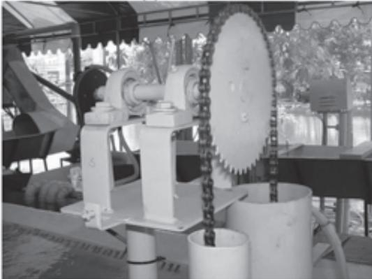
(c) Floating type water level connected to potentiometer
