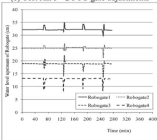
(e) Test run 5 – 4 FTO gate adjustments
