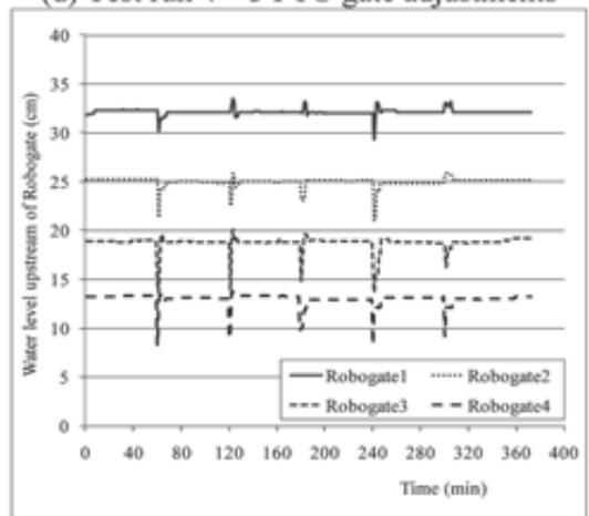
(f) Test run 6 – 5 FTO gate adjustments
