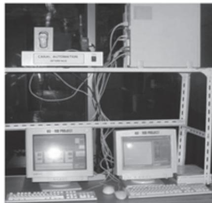
(e) Canal automation interface transferring the water level and gate position data between computer at master station and each Robogate via CB communication radio
