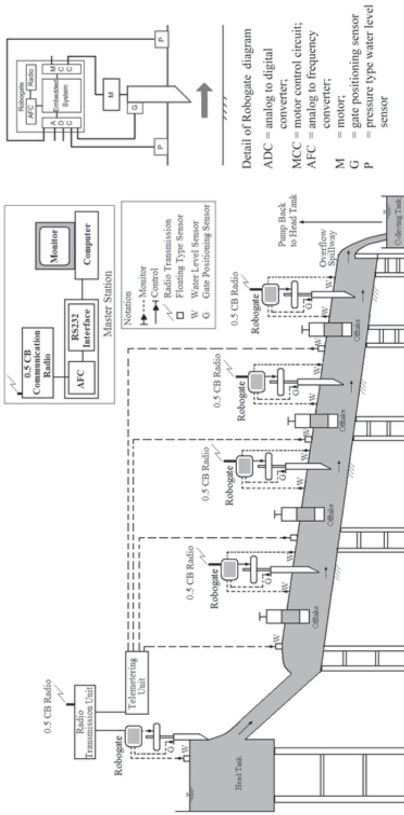
Figure 1 Diagram of canal automation model.
