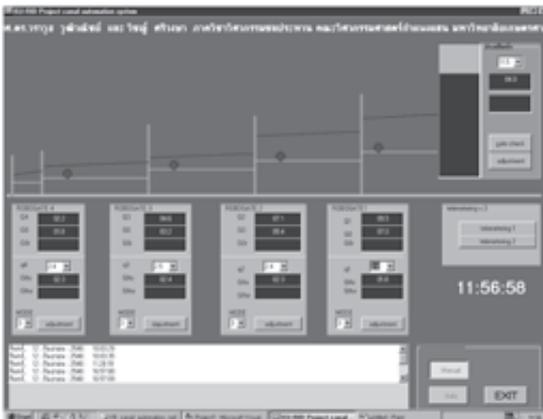
(d) Monitoring of water level and gate positioning in real-time operation at master station
