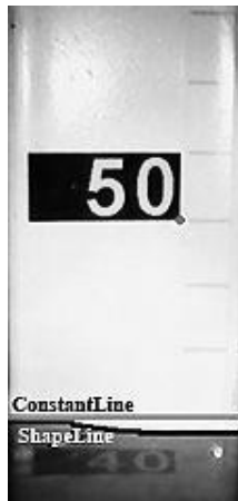
Figure 7. Water surface estimation methods, constant line and shape line
