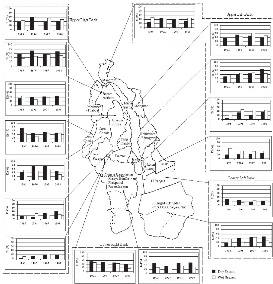
Figure 3 Irrigation efficiency of GCPP.
