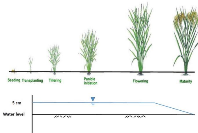
Figure 3: Schematic diagrams of water level controls for irrigation field in CF method
