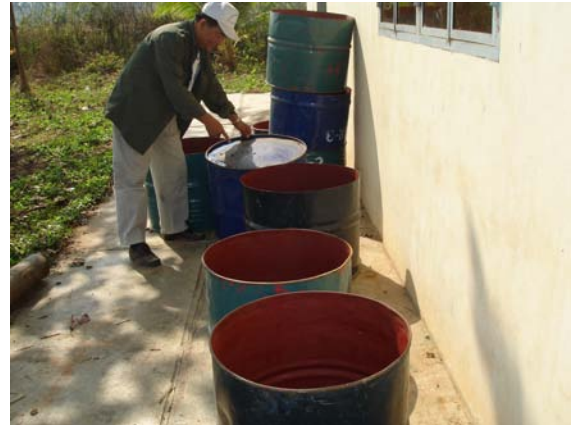
Percolation test tanks will be installed in paddy fields
