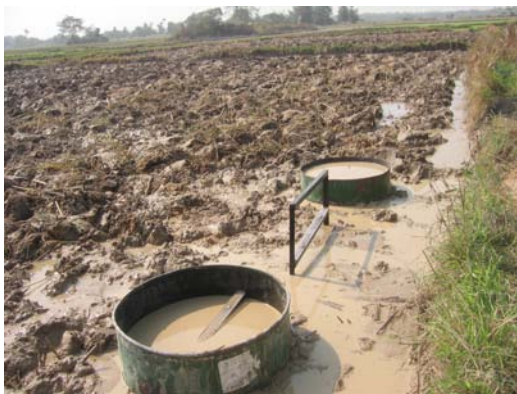
Equipment set for percolation in paddy field
