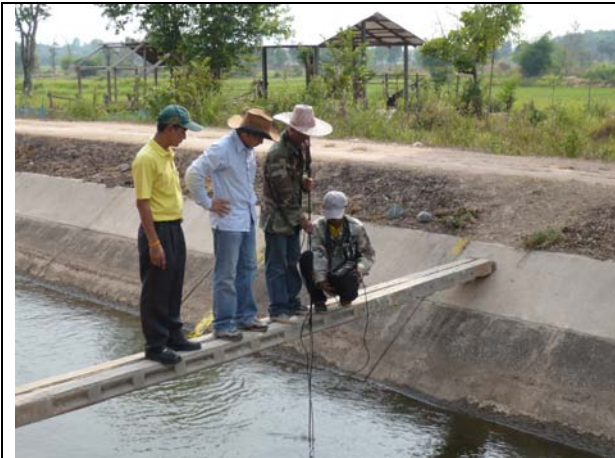
Checking flow conveyance test
