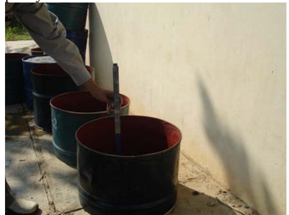
Percolation test tanks with reading scale
