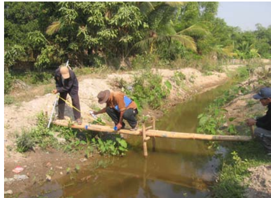
Make cross section and re-mark measurement point
