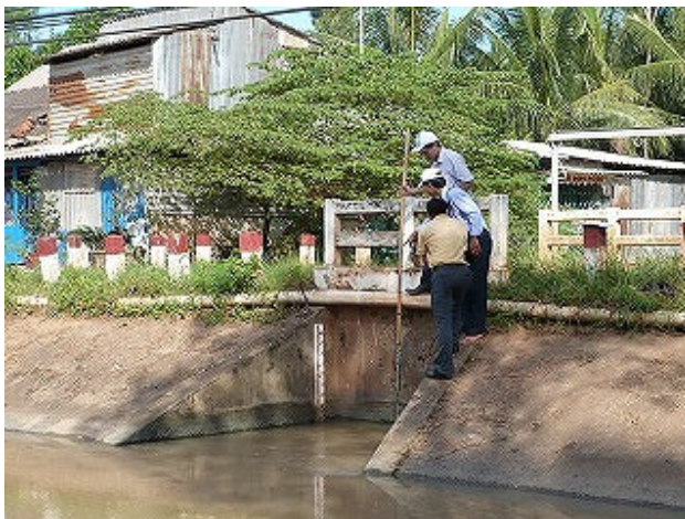
Conducting velocity for H-Q curve at HL 6 sulce
