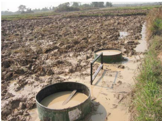
Percolation test in paddy field (during land preparation period, photo from last report)
