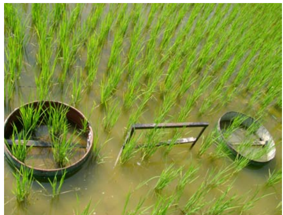
Percolation test in paddy field (2)
