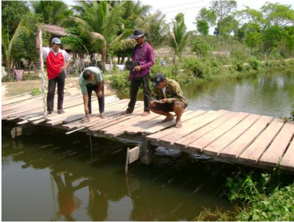
Flow conducting for conveyance test at main canal
