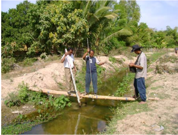
Conducting flow measurement at secondary canal
