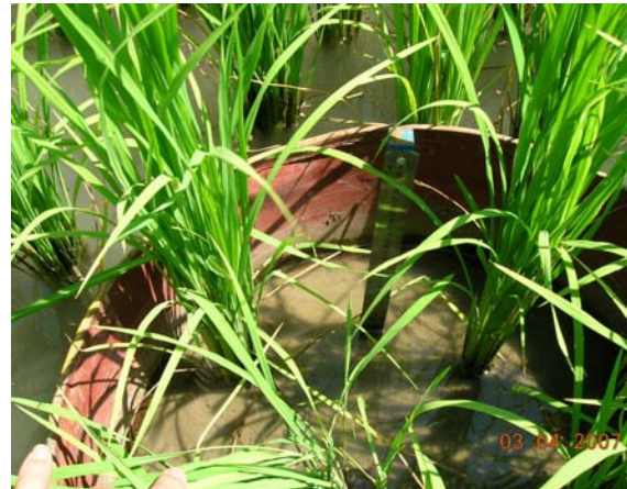
Scale or ruler installed inside percolation tank
