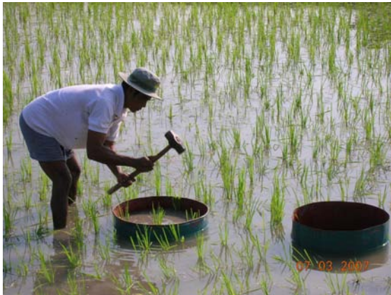
Farmer installed percolation test tanks
