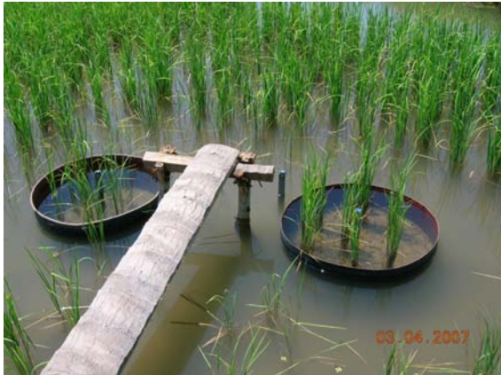
Set of percolation test during this field visit
