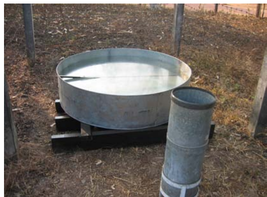
Evaporation and rainfall tanks at reservoir (project office)
