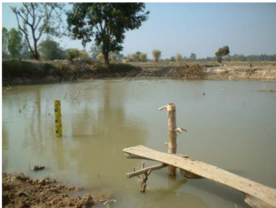
Percolation staff gauge installed in fishpond
