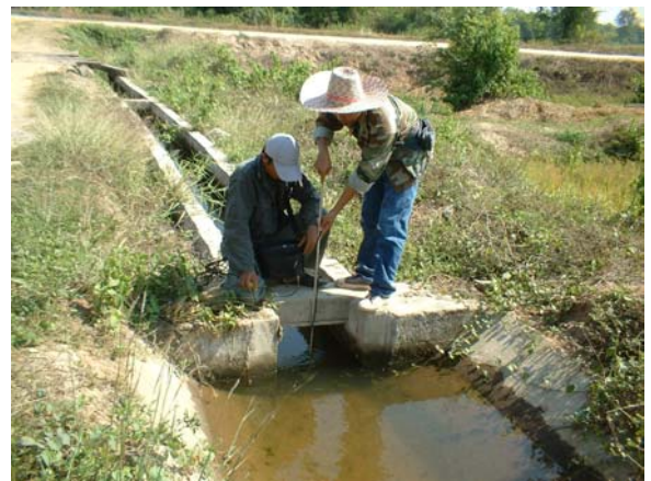
Measurement and calculation water discharge in the canal in order to check loss in the irrigation system for calculation of conveyance efficiency
