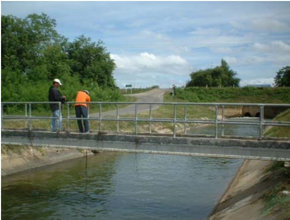
Measurement and calculation water discharge in the canal in order to check loss in the irrigation system for calculation of conveyance efficiency
