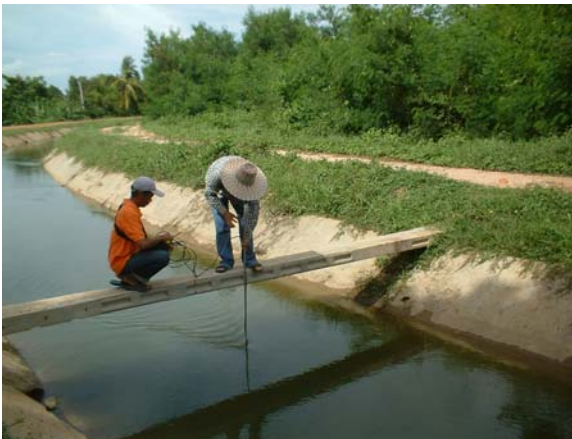
Measurement and calculation water discharge in the canal in order to check loss in the irrigation system for calculation of conveyance efficiency
