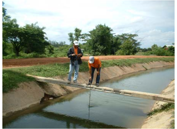
Measurement and calculation water discharge in the canal in order to check loss in the irrigation system for calculation of conveyance efficiency
