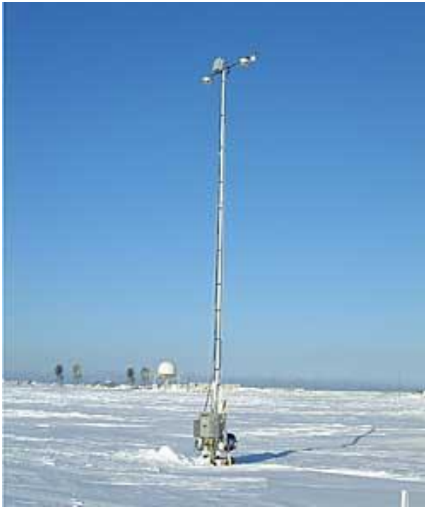
Ground Radiometers on Stand for Upwelling Radiation.
